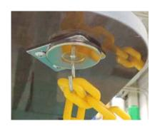
(14)Attach the magnet hanger to the main body of the machine, and hang the chain on it.
